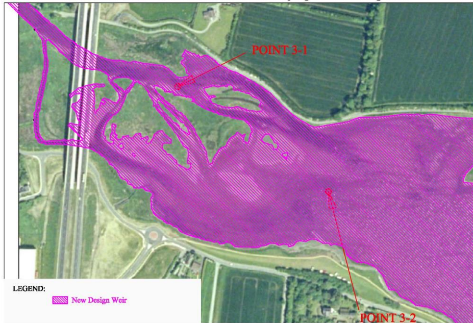
Malahide Viaduct Reinstatement - Water surface at spring low - New Design Weir
